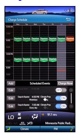
Another way of prolonging battery life is to schedule charging for later, rather than having start immediately. The delay allows the battery to cool in the meantime, a process referred to as "cold soak".
