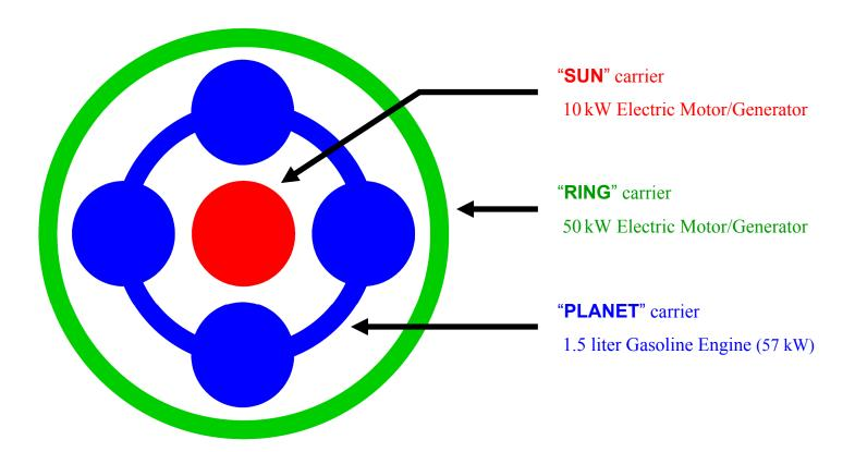
Prius doesn't actually have a transmission, because there are no gears and the power carriers are permanently engaged. The illustration you see above is a simplified diagram of what Prius has for the transfer of power instead. It very closely resembles another component found in all vehicles, a differential. The only difference is that there are multiple sources of power, rather than just one; hence the name "Power-Split-Device". To keep references simple, it can be called: "PSD".
